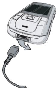
The battery symbol indicates the state of charge. During charging, the 4-bar charge indicators scroll; the maximum charge time for empty battery is 3 hours for a standard charger. When all four bars are steady, the battery is fully charged. You can then disconnect the charger. Depending on the network and condition of use, talk time goes up to 4 hours and stand-by time up to 300 hours.
