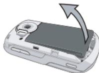
If your SIM card is delivered in a credit-card size, remove it from its holder and insert it under the metal clip holder, until it stops. Make sure that the clipped corner of the card is in the correct corner and that the gold contacts are facing down.
