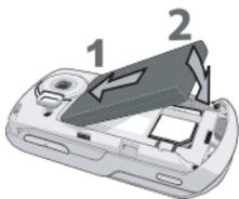
Replace the back cover by pushing it down into its slots, until it stops.
