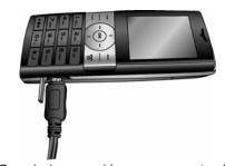
Once the battery and battery cover are installed, you can charge the phone. Plug in the connector as shown below. Then plug the other end into an AC power socket.
