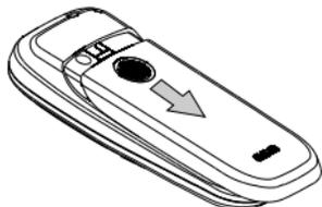
3. Hold the latch to lift up the battery.
