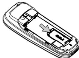
5. Slide the battery back (with the connectors facing downwards), until it stops.
