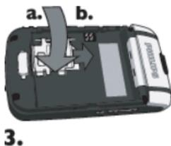
Slide the battery back into its slot, gold contacts downwards, until it stops. Then lock it by pushing it downwards. Replace the back cover by sliding it into its slots until it stops.
