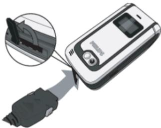
The battery symbol indicates the state of charge. During charging, the charge indicators will scroll; it takes around 2.5 hours to fully recharge your mobile phone. When all the scroll bars are steady the battery is fully charged. You can then disconnect the charger. Depending on the network and condition of use, talk time goes up to 8.5 hours and stand-by time up to 850 hours.
