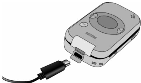
The battery symbol indicates the state of charge. During charging, the charge indicators will scroll; it takes around 2.5 hours to fully charge the battery. When all the scroll bars are steady, the battery is fully charged. You can then disconnect the charger. Depending on the network and condition of use, talk time and stand-by time can go up to 4 hours\* and 300 hours\* respectively.
