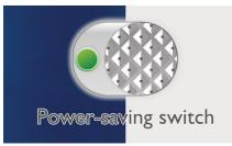
This Power-saving switch may well be the most convenient feature on your Philips mobile phone. By clicking the button located on the side panel, you can enable this function to help preserve your phone battery. It will shut down the WiFi, GPS and Bluetooth functions, while dimming the screen display simultaneously. Besides avoiding the multiple clicks needed to do likewise on other phones, this clever yet convenient button is definitely a lifesaver for heavy phone users.
