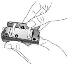
*When inserting the battery, be careful not to damage the metallic connectors of the SIM card slot.*
