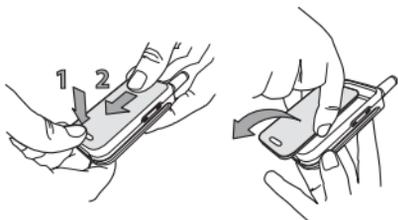
2. Remove the battery by pressing the inner clips one after the other, then pulling the battery from the left handside.
