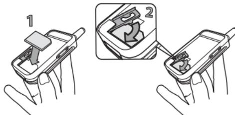
4. Replace the battery in its slot as shown below: first place its right side against the right edge of the phone and press until it clips.
