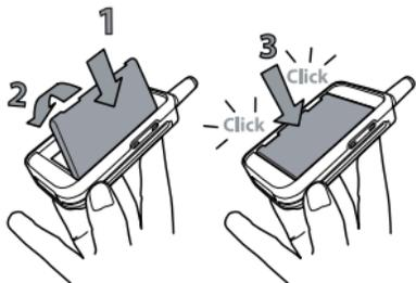
5. Slide the battery door into its slots, metallic connectors downwards, until it stops.
