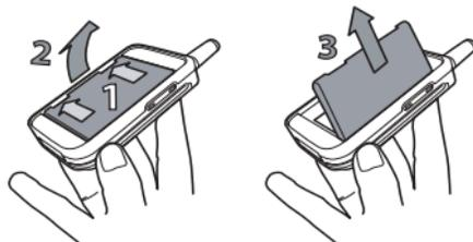
3. Remove the SIM card from its holder and place it on its slot (be careful that the clipped corner of the card is in the appropriate corner). Then push the plastic clip holder, until it stops and maintains the SIM card.
