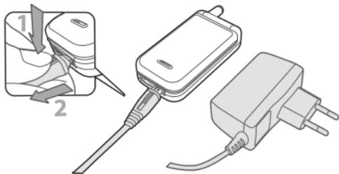
2. Plug the transformer unit into a main AC power socket with easy access. The battery symbol indicates the state of charge:
