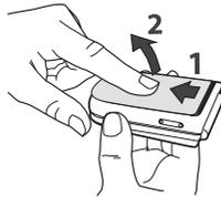
2. Remove the SIM card from its holder and insert it under the metal clip holder, until it stops. Be careful that the clipped corner of the card is in the correct corner.
