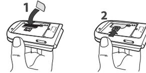
3. Place the battery in its slots as shown below: first place its right side against the right edge of the phone and press until it clips.
