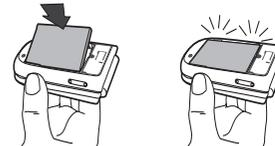
4. Replace the back cover of your phone: hook the front housing onto the hinges on the top of the phone, then press the bottom down until the latch catches.
