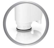
The water filter settings can be adjusted to the hardness of your water. Simply turn the adjustment ring on the Intenza+ water filter. Set it to A for soft water areas, B for medium water hardness (factory setting) or C for hard water. This will ensure optimal limescale protection and best taste.
