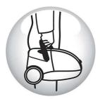
This vacuum cleaner has not one, but two carrying handles. When it is on its wheels, there is a handle on top which enables you to easily move the cleaner around with very little bending. The second handle on the front side of the appliance enables you to comfortably carry it around in an upright position.
