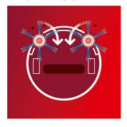
Side brushes and a vacuum remove dirt and dust from your floors. The exhaust filter traps fine dust and particles. It captures dirt and dust.
