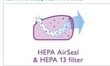
This Philips vacuum cleaner has been designed in such a way that all the air taken in is passed through the washable HEPA 13 filter (99.95% filtration) before it is exhausted. No escape is possible.
