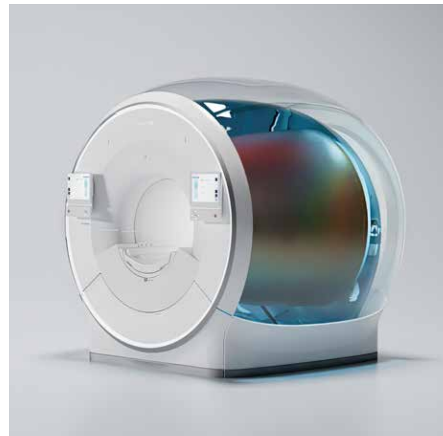
Classic magnet technology - ~1,500 liters of liquid helium
