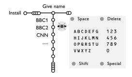
It is possible to change the name stored in the memory or to assign a name to a TV channel or external for which a name has not yet been entered. A name with up to 5 letters or numbers can be given to the channel numbers 0 to 99.
