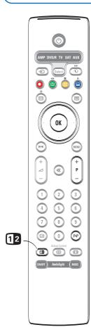
Press the 12 key to switch on **Dual screen**, **PIP** or one of the PIP modes according to the format selection made in the PIP format list in the General menu. See Setup, General, p. 7.
