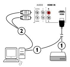
HDMI is the leading new standard for Digital High Definition video and audio interconnection. Eg. with a Digital Set top box, with HDMI-equipped devices like a PC, DVD-R, AV receiver...
