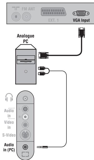
Connect the monitor output of your computer to the **PC VGA In** of the TV.
