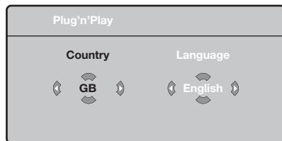
**⚠** If the menu is not displayed, press and hold down the  $\Delta+$  and  $\Delta-$  keys on the TV set for 5 seconds to display the menu.
