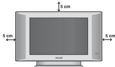
Place your TV on a solid stable surface. To avoid danger do not expose the TV to water, or a heat source (e.g. lamp, candle, radiator). Do not obstruct the ventilation grid at the rear.
