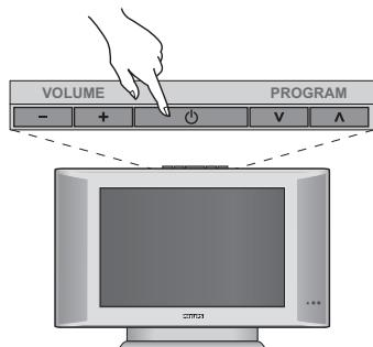
To switch on the set, press the on/off key. A green indicator comes on and the screen lights up. Go straight to the Quick Installation chapter. If the TV remains in standby mode (red indicator), press the P + key on the remote control.
