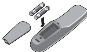
Insert the two R6-type batteries supplied, making sure they are the right way round.
