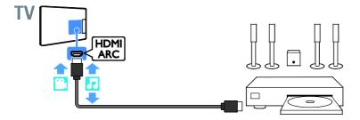
Connect the home theater with an HDMI cable and a coaxial audio cable to the TV.
