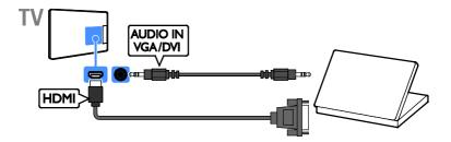
Connect the computer with a VGA cable and an audio cable to the TV.
