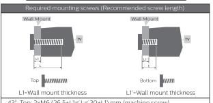
43": Top: 2xM6 (26.5+L1<L<30+L1) mm (machine screw)
