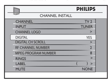
**3** Press ▼ to set the **RF CHANNEL NUMBER** to the physical channel number.
