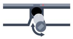
To replace the battery, rotate the small lid to the left to open
