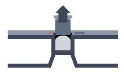
To replace the battery, press the small knob on the battery lid and slide the lid up to open. Replace the battery: type CR2032 (3V). Make sure the + side of the battery is visible. Replace the lid and slide it down until it clicks.
