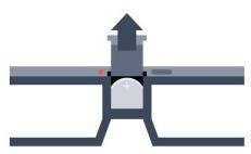
To replace the battery, press the small knob on the battery lid and slide the lid up to open. Replace the battery: type CR2032 (3V). Make sure the + side of the battery is visible. Replace the lid and slide it down until it clicks.
