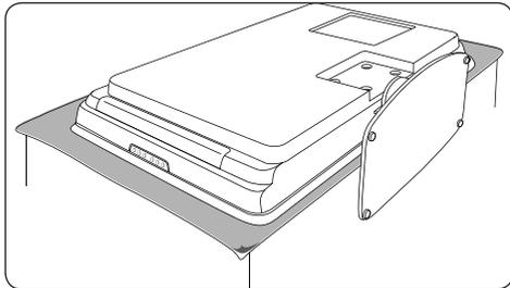
2. Using a cross-head screwdriver (not supplied), unscrew the four screws that secure the stand to the TV.
