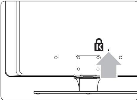
If connecting an anti-theft Kensington lock (not supplied), position the TV within reach of a permanent object (such as a table) that can be easily attached to the lock.
