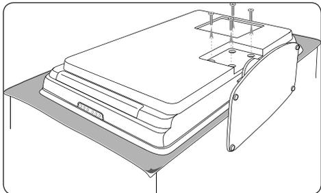
3. Firmly pull the stand from the bottom of the TV. Place both the stand and screws in a secure location for future reinstallation.
