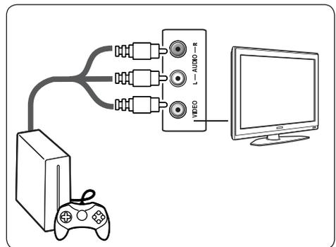
A permanent game console or camcorder can be connected to an HDMI connector or **AV IN** (component) connectors at the back of the TV.
