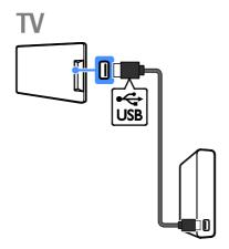
Connect the USB flash drive with a USB cable to the TV.
