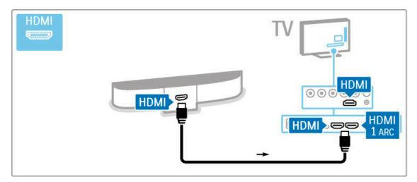
If you do not use the HDMI-ARC connection, add a digital audio cable (optical).
