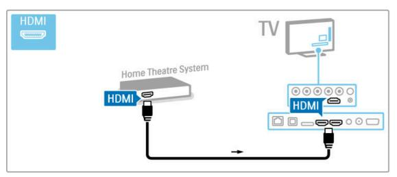
If you do not use the HDMI-ARC connection, add a digital audio cable (optical).
