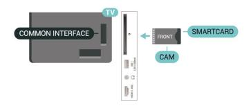
When you switch on the TV, it may take a few minutes before the CAM is activated. If a CAM is inserted and subscription fees are paid (subscription methods can differ), you can watch the scrambled channels supported by the CAM smart card.
