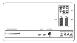
There is a wide range of audio and video equipment that can be connected to your TV. See 'To make video and audio connections', p. 43. **EXT1** can handle CVBS, RGB and Audio L/R; **EXT2** can handle CVBS, S-VIDEO, RGB and Audio L/R;
