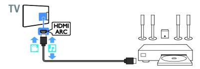
Connect the home theater with an HDMI cable and a coaxial audio cable to the TV.
