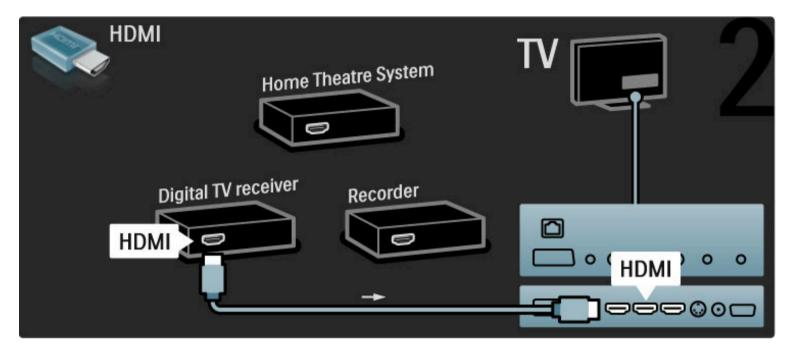
Then use an HDMI cable to connect the Disc Recorder to the TV.
