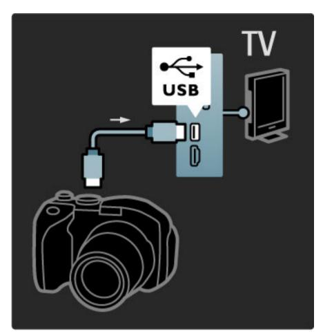
If the list with the content of the camera does not appear automatically, your camera might need to be set to transfer its content with PTP (Picture Transfer Protocol). Read the user manual of the digital photo camera.
