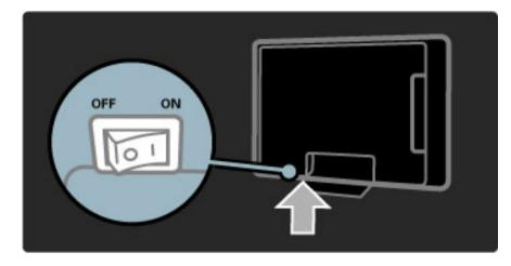
If the red indicator light is off, switch on the TV with the power switch.
