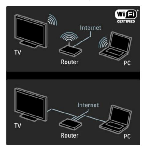
If you use a wired connection to the router you need a network (Ethernet) cable.
