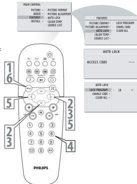
Note:You can block additional channels by using Number buttons to jump to another channel.
