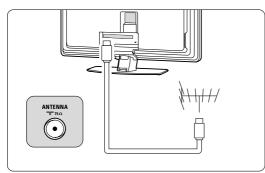
**1** Locate the antenna connection at the back of the TV.
