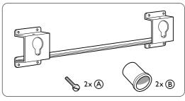
**2** Insert just a little bit both security screws in the wall mount bracket.
