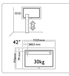
6 Position and level the wall mount bracket and fix the bracket firmly to the wall.
