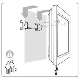
Secure the TV in the bracket by screwing in the 2 already fitted screws (A).
