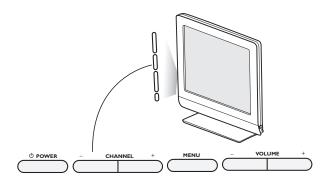
Should your remote be lost or broken you can still change some of the basic settings with the buttons on your TV. Press the power switch () to switch the TV on.
