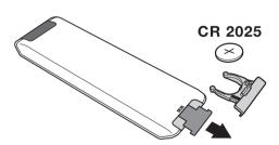
Pull out the plastic insulation sheet from the battery, this will activate the remote control. The battery supplied with the appliance does not contain mercury or nickel cadmium so as to protect the environment. Please do not discard your used batteries, but use the recycling methods available (consult your distributor).
