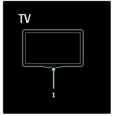
1. Ambient sensor / remote control sensor Ambient sensor is available on certain models only.
