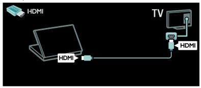
Connect the computer with a DVI-HDMI cable to the TV.
