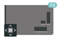
1 - With the TV switched on, press the joystick key on the back of the TV to bring up the basic menu.
