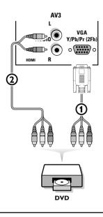
Connect the device with **2Fh YPbPr** output to the **VGA** connector ① (with the supplied adapter cable VGA to cinch) and to the **L** and **R AUDIO** jacks ② of **AV3**. See also the manual of your High Definition device.
