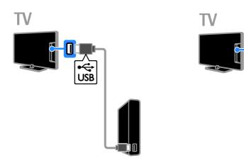
Connect the USB hard drive to the TV with a USB cable.
