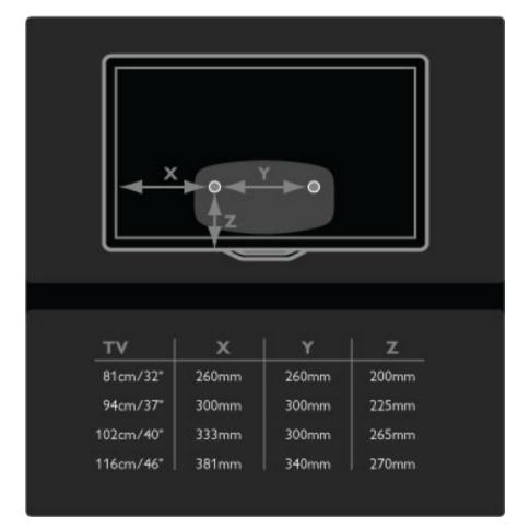
Fix the 2 mounting discs. Use screws with a diameter of max 6mm.
