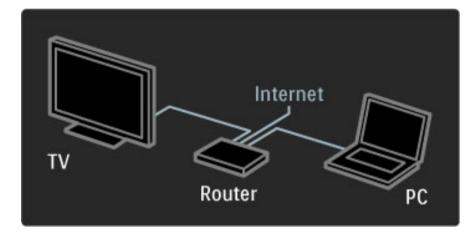
If you use a wired connection to the router you need a network (Ethernet) cable.
