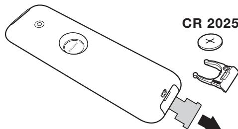
Pull out the plastic insulation sheet from the battery, this will activate the remote control. The battery supplied with the appliance does not contain mercury or nickel cadmium so as to protect the environment. Please do not discard your used batteries, but use the recycling methods available (consult your distributor).
