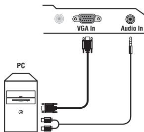
Connect the monitor output of your computer to the **PC VGA In** of the TV.
