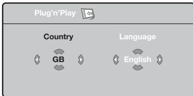
If the menu is not displayed, press and hold down the **▲-** and **▲+** keys on the TV set for 5 seconds to display the menu.
