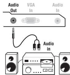
To connect to a hi-fi system, use an audio connection cable and connect the sound output **Audio out** on the TV set to the "AUDIO IN" "L" and "R" input on your hi-fi amplifier.
