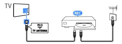
Connect the recorder with a composite cable (CVBS) and an audio L/R cable to the TV.
