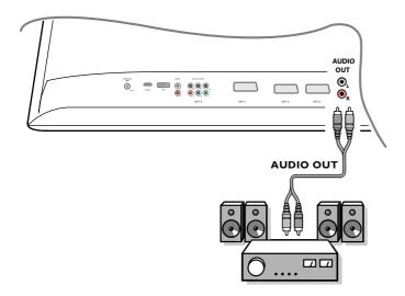
Connect an analogue MultiChannel Surround receiver to the  $AUDIO\ OUT\ L$  and R connectors at the bottom of the TV. The volume has to be controlled via the MultiChannel Surround receiver.
