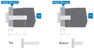
L1=Wall Mount thickness L1'=Wall Mount thickness
