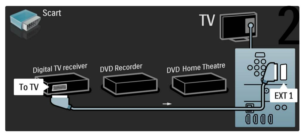
Then use 2 Scart cables to connect the Digital receiver to the DVD Recorder and the DVD Recorder to the TV.
