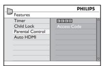
Key in the access code 0711 by using the 0 to 9 digit keys. The word Incorrect appears on the screen.
