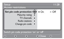
Press the ◀ or ▶ key to select On, and press the OK key to exit.
