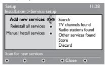
A search begins. Any new channels are added to the channel list menu. The percentage of the installation that has been completed and the number of channels found is displayed.
