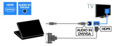
Connect the computer to the TV with a VGA cable and an audio cable.
