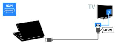
Connect the computer to the TV with a DVI-HDMI cable and an audio cable.
