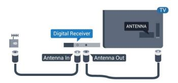
Next to the antenna connections, add an HDMI cable to connect the Set-top box to the TV.
