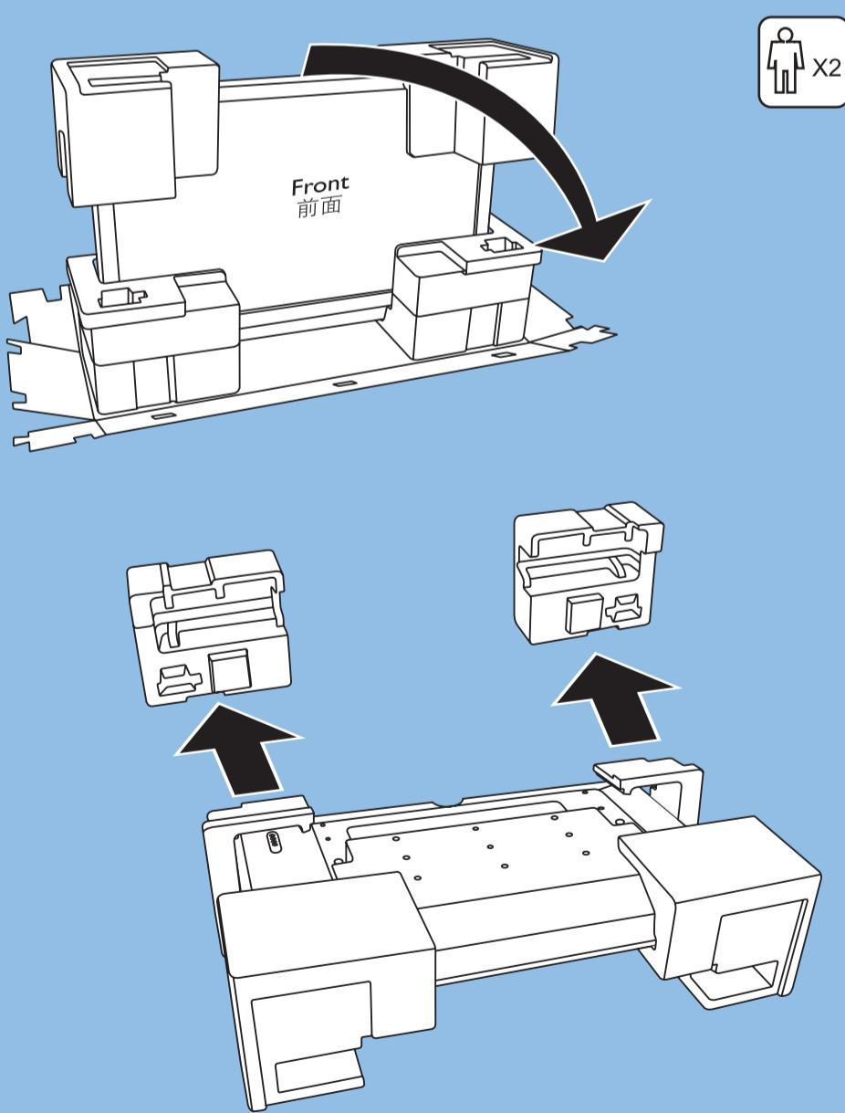
Remove base accessories from the box and fix the frame with the base.
