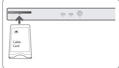
To receive scrambled DTV signals you will need a CA (Conditional Access) module and a Smart card provided by the service provider.
