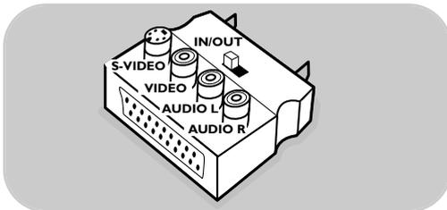
**Note:** Use the scart to cinch adaptor (with the switch in the **IN** position) to connect (temporary) peripheral equipment to **EXTERNAL 1** or **2**.
