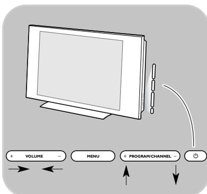
In case your remote is lost or broken, apart from channel selection and volume adjustment, you can still change some of the basic settings with the keys at the side of your TV.
