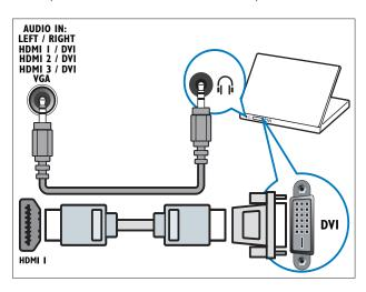
HDMI cable and HDMI-DVI adaptor (side HDMI and AUDIO IN L/R)
