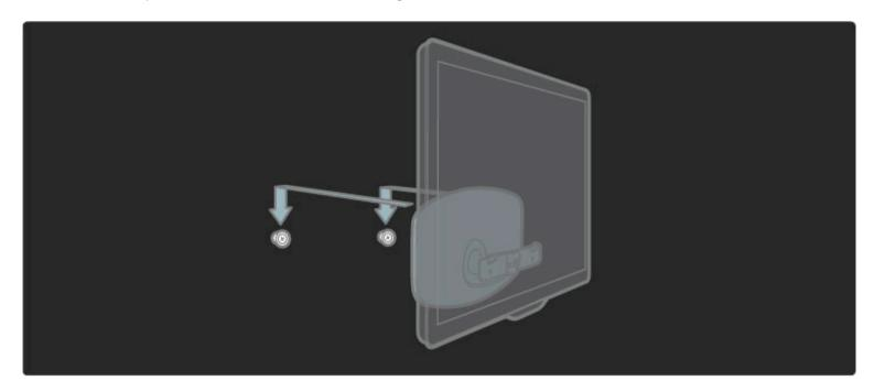
To level the TV, pull the bottom of the TV towards you slightly and let it slide on the discs.
